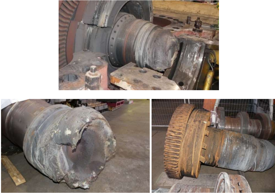
Figure 40 HP turbine, LP turbine and generator shaft damage
